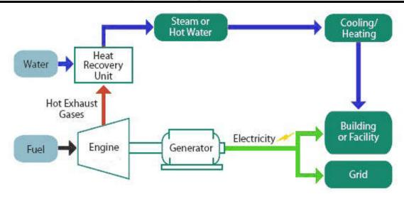
We offer Combined Cooling Heating and Power (CHP and CCHP) packages for our gas generator sets. It can recover 75%-90% combined electrical and thermal efficiency, resulting in major reductions in your overall energy costs. In the past years we have supplied CHP systems to Germany, Russia,Indonesia etc. We have the experience and capabilities to meet your total energy requirements.
